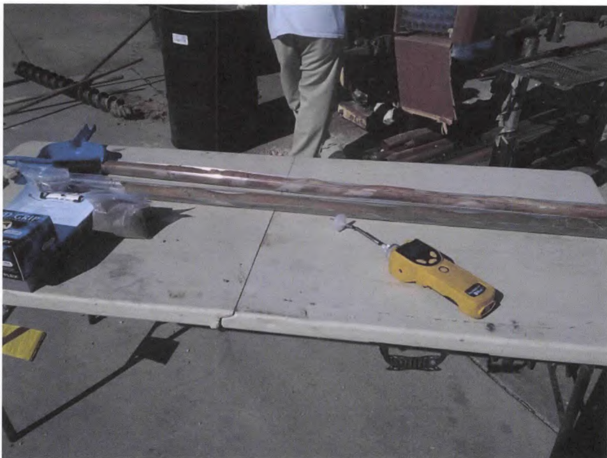
Cores analyzed with Photoionization Detector.
