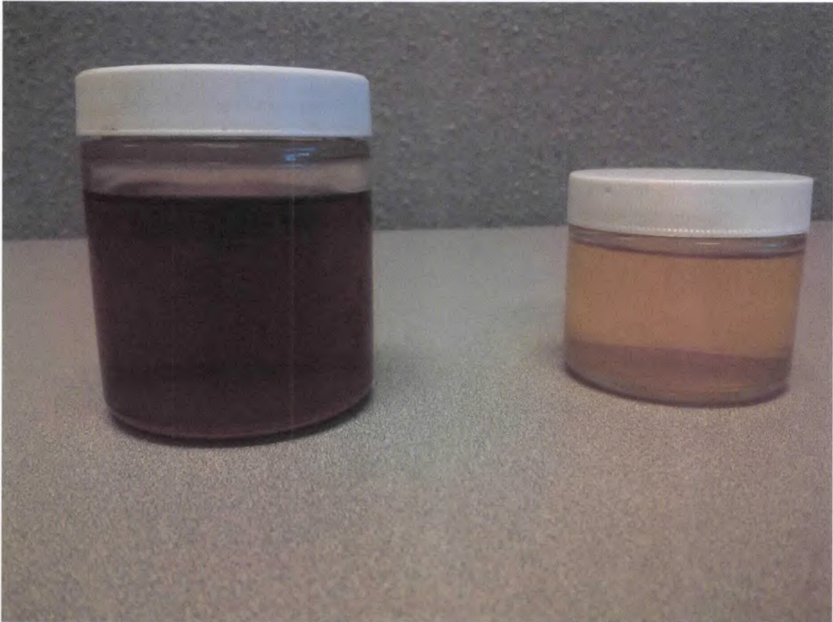
Aged/weathered LNAPL from recovery event at the Site on left. Fresh diesel on right for comparison only, not from Site.
